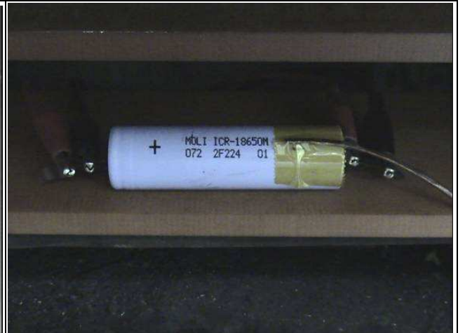
T8: Forced discharge Test
