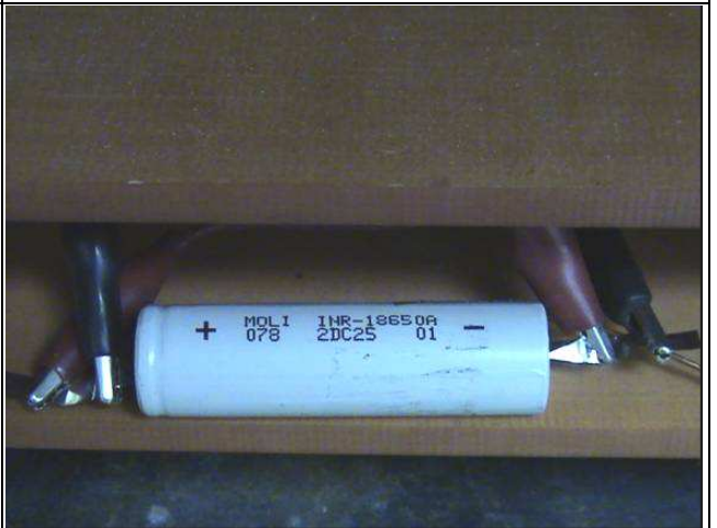
T8: Forced discharge Test
